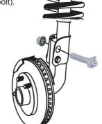
on bolt, into the strut housing in the same direction the OE bolt came out.
