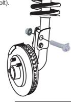
Install adjusting cam, with the washer already on bolt, into the strut housing in the same direction the OE bolt came out.
